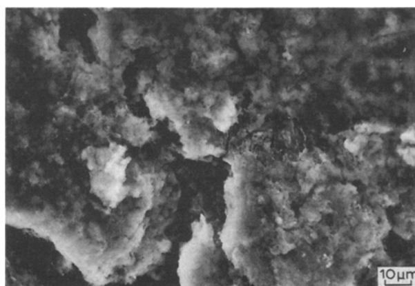
Fig. 8. SEM photograph of Li-B alloy electrode surface: anodically polarized at 10 \text{ mA cm}^{-2} for 10 min.
