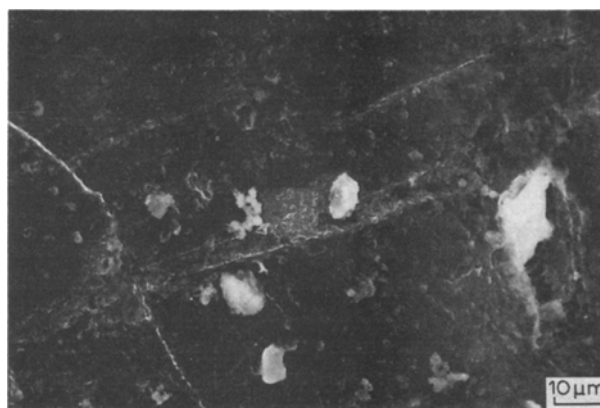
Fig. 7. SEM photograph of Li-B composite electrode surface: anodically polarized at 10 \text{ mA cm}^{-2} for 10 min.
