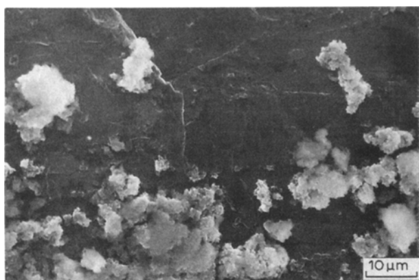
Fig. 6. SEM photograph of lithium electrode surface: anodically polarized at 10 \text{ mA cm}^{-2} for 10 min.
